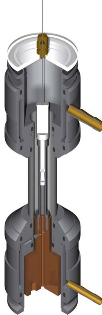
Figure 4.2: Schematic construction of the PAC-furnace [ARE10]. The sample is fixed on a sample holder (white) which is placed in the graphite heater.
